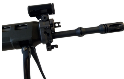
Figure 9: Guidon annulaire Zumkeller
